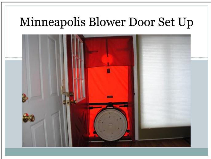
Install frame cross bar to support fan
