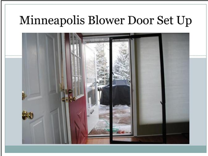
Assemble Frame, rough size frame into door opening, outdoor pressure hose is placed away from fan (around a corner)
