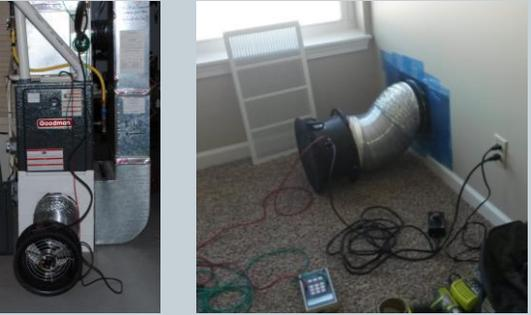
Photo 1 – Duct blaster connected to air handler
