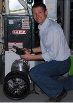
Duct Leakage Testing – “Duct Blaster”
