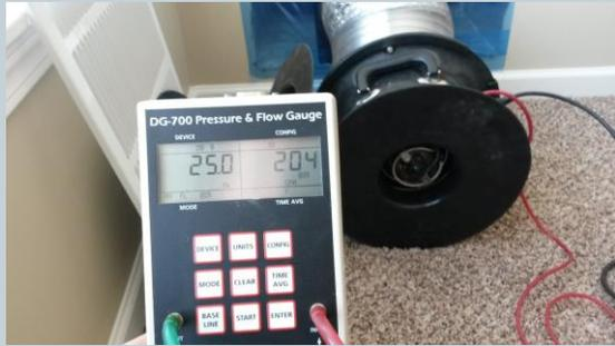
25 Pa is the pressure of the ductwork
