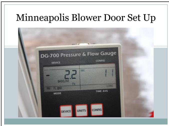
Turn on manometer and set Manometer to "PR/ FL@50" then hit "baseline"
