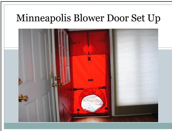
Install door and lock cam's to tighten the fit
